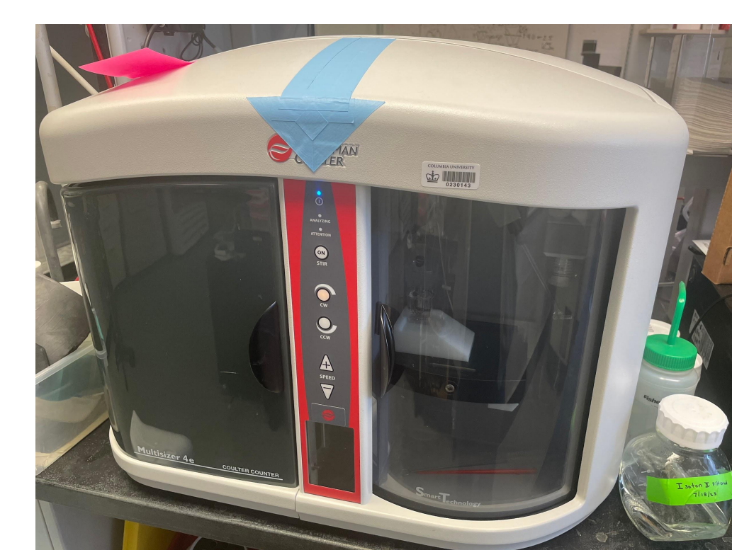
Figure 3. Multisizer 4e Coulter Counter Throughout the entire experiment, a sizing machine was utilized daily, and it was cleaned using Isoton II. The sizing machine employs electrical zone sensing (EzS) technology for its measurements.
