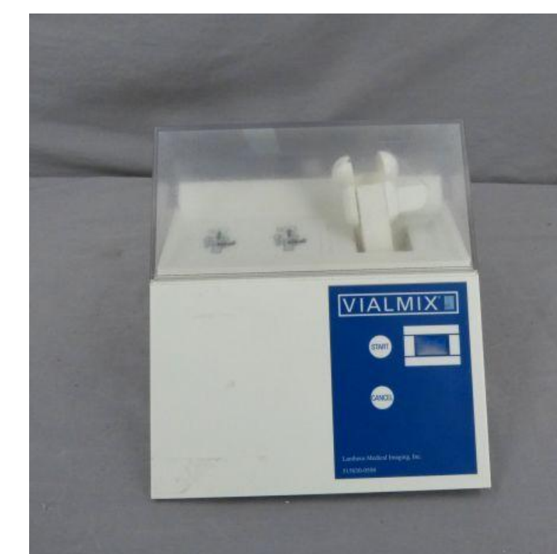
Figure 4. Vialmix®. The Vialmix pictured is used for standard activation of microbubbles.
